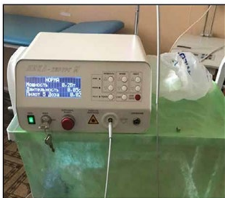
Fig. 3. LIKA surgeon HeNe laser (with a fiber optic light guide) for exciting fluorescence with 630-633 nm light
